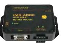
The IMS-4310 Dual Relay Output Module allows you to control two devices from any IMS-4000 Host or Node. Each output may be controlled either manually or automatically. Each output has the option of providing either a dry relay contact or 12VDC power. Two switches located inside the device select the output type.
