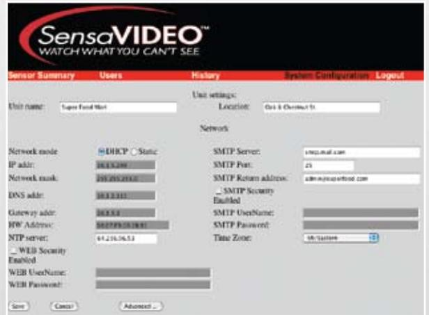
Configuration for the SensaVideo is performed through a built-in web page. Just browse to the address of the product on your local network to have full access to all programming options. You can configure your sensor types, names, alarm limits, recognition times, notification responses, and more.
