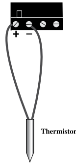
Wiring a Temperature Sensor
